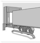
This visual aid makes it easier to park the vehicle and reduces the risk of collision. Especially advantageous for docking stations with wide leveller lips and cushion shelters. Parking guides can be bolted or cast in concrete on the floor before the leveller.
