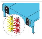
Crawford Dock-IN White & Red is the optimum combination of both systems for easy and safe docking. The white LEDs provide the visual target and the red LED positions the truck at the right distance to the dock. The white guiding LEDs turn off when the truck is detected and at the same time the red LED turns ON. Crawford Dock-IN White & Red guide the truck driver in the best possible way for an easy and safe docking.
