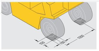
In the drawing measures for a leveller with a load capacity of 60kN are shown.
