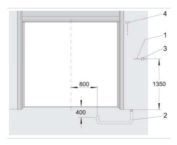
1 Mains supply: 3/N/PE AC 50 Hz 230/400V Mains fuse: D0 10 A gL Motor power: 0,75 kW
