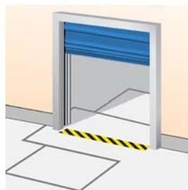
A sensor in the floor detects a metal object (usually forklift trucks, pallet trucks) and opens the door automatically. This is an ideal solution for frequent vehicle traffic. Installed on the outside, inside or both sides of the door in the ground.
