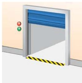
One or two sets of green and red lights indicating that the door is open or closed; continuous green light when the door is open, continuous red light when the door is closed, optionally flashing light when the door is moving or not fully open. Installed on the inside and/or outside wall beside the door.
