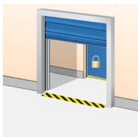
Developed for climate control or safety; if door A is open, door B cannot be opened. If door B is open; door A cannot be opened.
