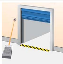
A hand-held radio transmitter allows door operation from a vehicle or any position within 50-100 meters from the receiver and aerial at the door. For closing, the door can be provided with a photocell beam. Receiver installed in control unit, antenna optionally installed on the wall beside the door.
